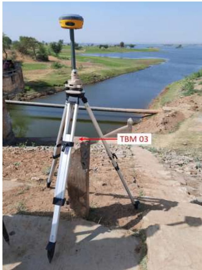
Figure 3.2: Temporary Benchmark (TBM 03)
